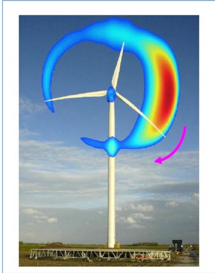
Figure 3 - Average distribution, over many revolutions, of the noise source distribution in the azimuthal plane, for a typical, modern, large-size WT, projected over a picture of the WT, for illustration purposes only (Oerlemans, Wind Turbine Noise: Primary Noise Sources, 2011)
